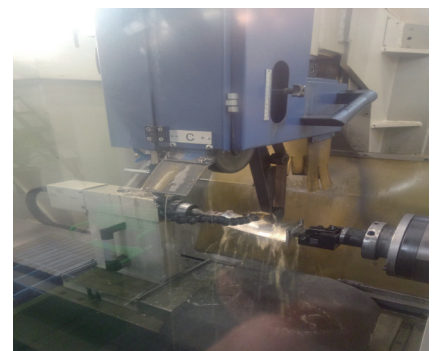
图9 砂带抛光叶身型面 Fig.9 Type abrasive belt polishing blade body surface
